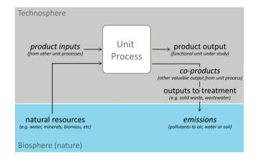
Figure 3 Inputs and outputs of a unit process in CFP.
